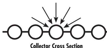
SUNHEATER collectors have a web construction designed for maximum heat absorption regardless of the position of the sun.
