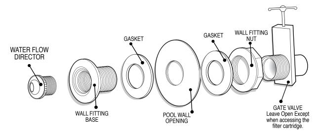
IMPORTANT FLOW TIP: The gate valves can be partially shut to control water flow. The further openings for the water return and sometimes receive less pressure. Slightly reducing the gate valve openings nearest to the pump maintains even pressure.
