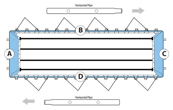
Continue inserting them through the shorter pool wall sleeve. Also attach the u-pipes and verticals. These walls will not need to be anchored up., as the anchored longer walls will hold them up.
