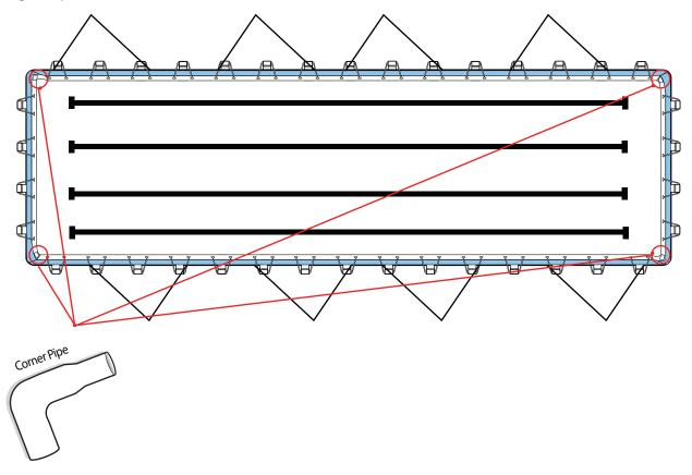
**WARNING**: All the frame components are designed to slip into place. If they are not going in, it is because the connections are not straight or the liner is bunched up.
