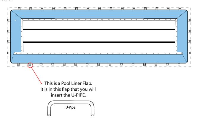
Once the horizontal pipes and u-pipes are in place, you can start attaching the vertical pipes. There is two per u-pipe. They fit over the u-pipe and through the top liner sleeve openings into holes on the horizontal pipes.
