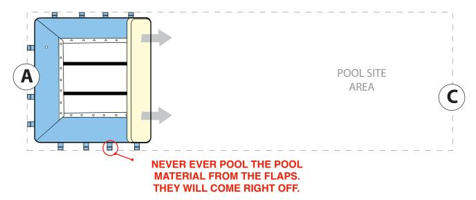
After unfolding, you can now start to position the pool material in the proposed pool site. Again, creating gentle waves to trap air to move the material. Again, NOT BY USING THE FLAPS.
