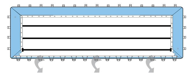
Once the pool wall is upright (90° from the ground), you will need to anchor the pool wall temporarily to hold it in place. This anchoring will remain in place until the pool is filled. We will explain why later. The rule is to have a secure anchor, able to hold at least 50 funds, every 10 feet. The rope/strap can slip around the exposed horizontal pipe found at the sleeve openings every five feet.
