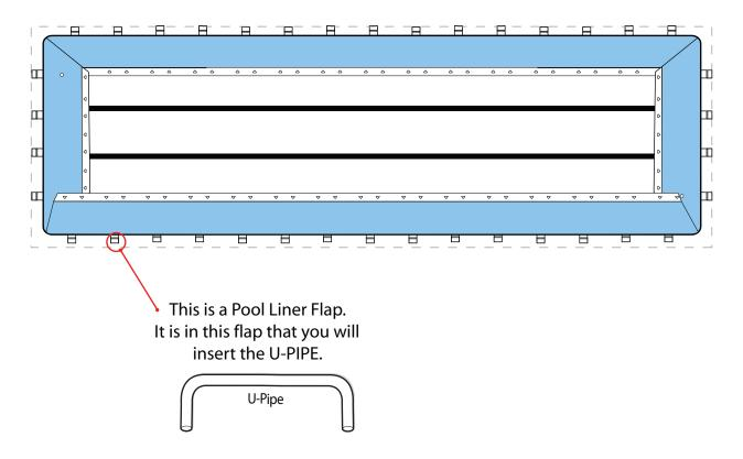
Once the horizontal pipes and u-pipes are in place, you can start attaching the vertical pipes. There is two per u-pipe. They fit over the u-pipe and through the top liner sleeve openings into holes on the horizontal pipes.
