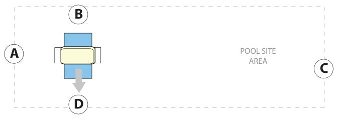
Remove the steel poles used with the carrying case and discard - you will not need them for the pool. Unfold half the liner towards side D, then fold the other half towards side B. You can now remove the carrying case form underneath the liner.
