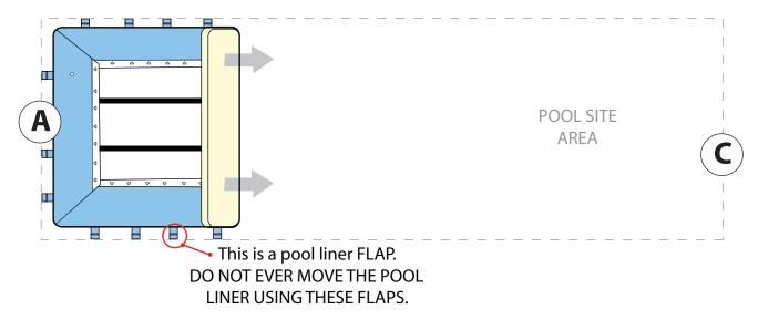
Finish unfolding the liner and position the pool liner accordingly. But remember, NEVER USE THE POOL LINER FLAPS TO MOVE THE LINER!!
