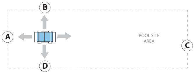
Open up the carrying case and inspect the liner. The fold opening in the liner should be facing side B of your pool site area, so that the first roll out of the folded liner would be towards side D. If this is not the case, you will need to rotate the liner.
