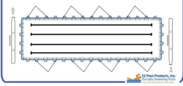
The corners are similar to the horizontal pipes in that they have a female and male side. They can be a bit stubborn to get into place, as they help to keep the pool frame taught. By maneuvering the liner material around and the frame you can get the corners in place. Once all four are in place, you can start filling the pool.
