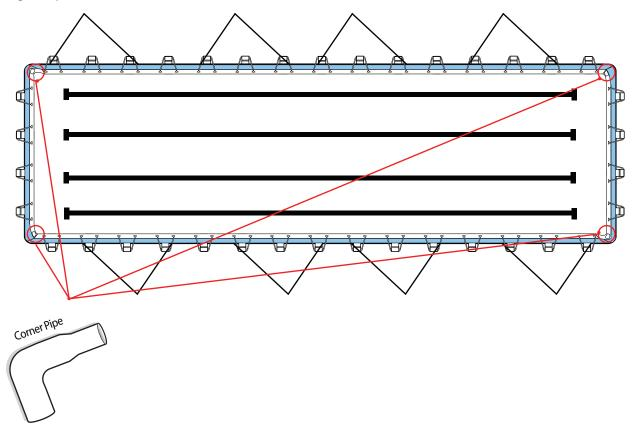
**WARNING**: All the frame components are designed to slip into place. If they are not going in, it is because the connections are not straight or the liner is bunched up.
