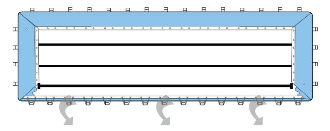
Once erected, use rope to anchor the pool wall up temporarily. For a pool wall this long, you should have at least 4 anchor points. There purpose is merely to hold the pool wall while we finish assembling the pool and filling it with water. Once filled, the anchor lines will go loose and can easily be removed.
