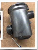
Located in a plastic bag is a black connector piece and two screws. Remove these two black connector parts, place them around the neck of the Hair/Lent pot and use the two screws to connect.
